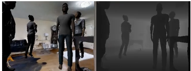
Figure 1. Dynamic obstacle augmentation adds several moving pedestrians as obstacles (visualized in RGB, left, and depth, right).
