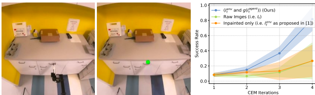
Figure 5. Real-world experiment setup and results. (left) Raw views from camera, (center) Agent-agnostic representation. (right) Success rate as a function of CEM iterations.
