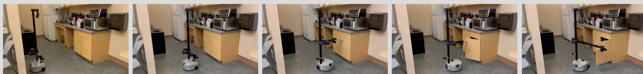
Figure 1. This paper presents a system for opening cabinets and drawers in novel real world environments using a commodity mobile manipulator. Here we visualize an example execution of our system interacting with a novel object in an unseen environment. We include the following frames: before navigation, after navigation, pre-grasp pose, during manipulation, and at the end of manipulation. We evaluate our system across 13 unseen environments from 10 distinct buildings for a total of 31 unique articulated objects in the real world.
