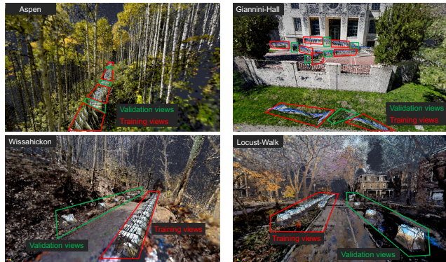
Figure 2. Top: Aspen and Giannini Hall scenes from Nerfstudio [1] contain validation views that are similar to training views. Although Splatfacto has good rendering quality on these data in Tab. 2, it does not accurately render dissimilar views in Fig. 1. Bottom: We created two new scenes, named Wissahickon and Locust Walk, where validation views are much more different than training views. For these new scenes, Splatfacto has a much worse validation PSNR than NeRF; see Tab. 2. All images above are rendered using Gaussian splats obtained from NeRF-SH without fine-tuning; this is called NeRFGS with zero iterations in Tab. 2.
