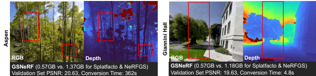
Figure 4. GSNeRF can be used for saving memory and editing the NeRF. We convert NeRFGS model, as in Fig. 3, back to NeRF-SH to get GSNeRF (Left). GSNeRF stores memory intensive GS models as more compact NeRFs. Also, GSNeRF with NeRFGS enables easy modifications to the scene represented by the NeRF by converting into a GS, modifying the Gaussians, and converting it back. As an example, we have edited out the lamp post from Giannini Hall in Fig. 1 through GSNeRF and rendered the image (Right) using NeRF-SH.
