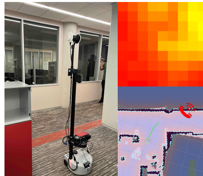
Figure 1. Our robot predicts an acoustic field with a frequency-adaptive model and navigates to locate the sound source.
