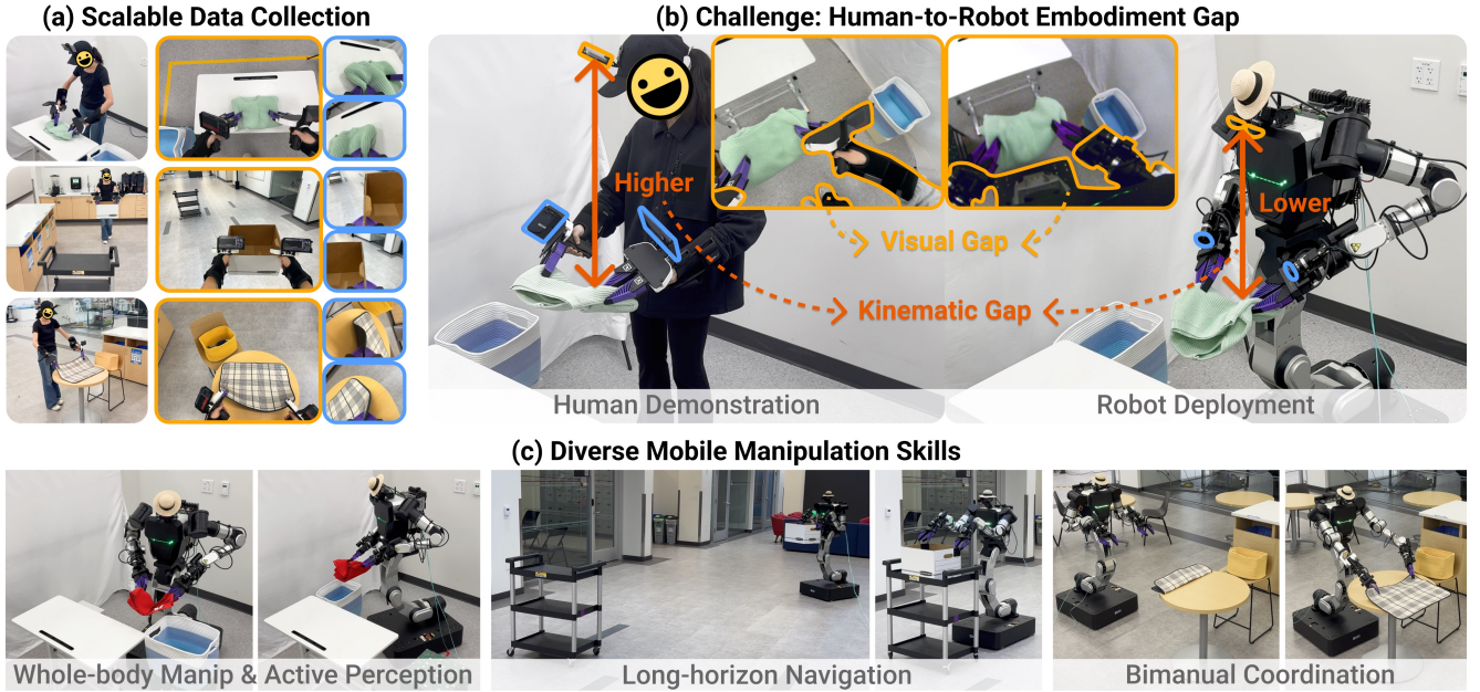
Figure 1. Whole-Body Mobile Manipulation Interface (HoMMI) . (a) We extend UMI with egocentric sensing to enable scalable mobile manipulation with active perception . (b) However, the new egocentric view creates a substantial embodiment gap in both observation and action space, making policy transfer difficult. (c) We bridge this embodiment gap by carefully redesigning the visual and action representations and integrating them with a constraint-aware whole-body controller. Together, HoMMI is able to learn diverse mobile manipulation skills directly from human demonstrations, without any robot teleoperation data.
