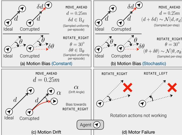
Figure 2. **Dynamics Corruptions.** We show the kinds of dynamics corruptions supported in ROBUSTNAV. Motion Bias (C & S) are modeled to mimic friction. Motion Drift models a setting where translation actions have a slight bias towards rotating right (or left). In Motor Failure, the one of the rotation actions fail.
